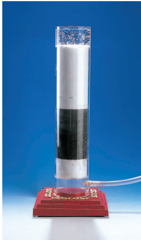
Insulation (Ext.) concrete, insulation (Int.) breathing model – blown air goes through three layers
