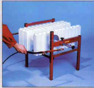
2. With the isorast saw or hot wire cutter, components are easily cut to size.
